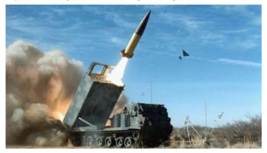
An ATACMS missile being launched from an M270 MLRS.
