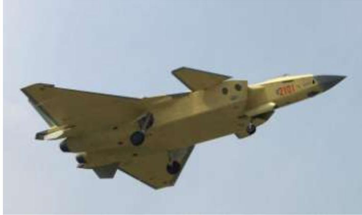
The 2101 aircraft is equipped with unique diamond-shape infra-red distributed aperture and electro-optical targeting sensors (under the fuselage) enabling the pilot to acquire air and surface targets in stealth mode, without using the powerful AESA radar.
