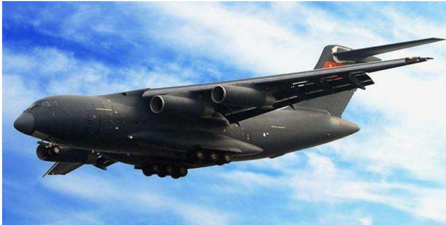
The first Xian Y-20 military transport aircraft was delivered to the People's Liberation Army Air Force (PLAAF) on June 15. Developed by Xian Aircraft Corporation, the Y-20 has an empty weight of 110 short tons, making it the largest military aircraft currently in production—larger than Russia's Ilyushin Il-76. Boeing's C-17 Globemaster III is bigger than the Y-20—the C-17's
