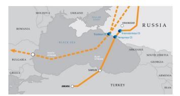
The total capacity of the planned gas pipeline, which has been unofficially dubbed the «Turkish Stream,» will be 63 billion cubic meters of gas per year, supplied via four legs. The pipeline will travel for 660 kilometers along the route planned for South Stream, and for another 250 kilometers along a new corridor toward the European part of Turkey.
