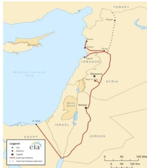
*Map (1) above: The Arab Gas Pipeline conceived to transport natural gas from Algeria, Libya, Egypt and Iraq has already been built through Syria. Plans are to complete the pipeline from Syria to Turkey where it will eventually connect to the planned Nabucco pipeline to deliver gas to Europe. Iran has recently expressed interest in connecting to the pipeline to run from Iraq. This is almost certainly the reason for the U.S. alliance with Iran to defeat IS. Source: EIA*
