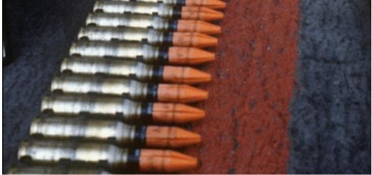
Mark 149 Mod 2 20mm depleted uranium ammunition for the Phalanx CIWS aboard USS Missouri. Photo: US Navy.
