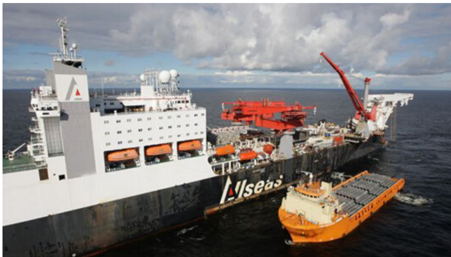
The Solitaire, a ship laying pipe as part of the Nord Stream gas pipeline project in the Gulf of Finland (Photo: archive.government.ru)
